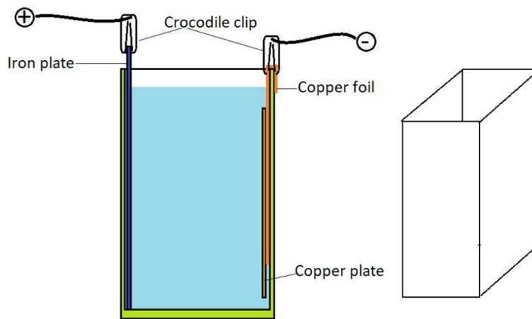
Set the output voltage of the power supply to a voltage a little higher than 2 V (i. e. 3 V) and the current to 0. If the distance between the iron and copper plates is too long, the voltage should be increased to reach the rated current. A distance of about 10 cm is ideal.
