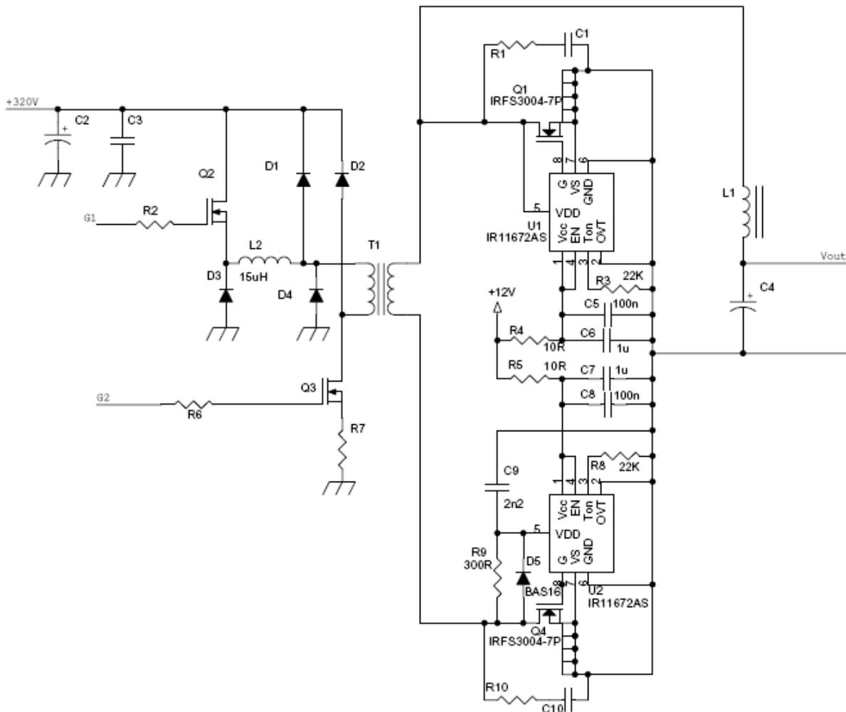
When Q2 and Q3 turn on, the current was flowing through Q1, acting as a free-wheeling diode. Because there is a delay time from U1 detecting the polarity change and Q1 switching off, for some nanoseconds Q1 short circuits de secondary.
