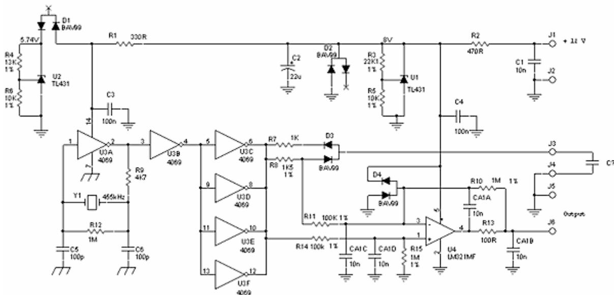
U3A is an oscillator using the ceramic resonator Y1. The output of U3C to U3F charges and discharges the capacitor to be measured at a 455kHz rate. The charge current flows through R8, and it is filtered and amplified by the differential amplifier U4. The discharge is made through D3. The average current in R8 is proportional to the capacitance.
